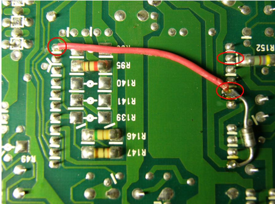
3. Remove Pin 14 (lower RHS) from the board and move to previously removed Pin 16 (upper RHS) and solder in. Reinstall Pin 11 (lower LHS) to the board using jumper wire or similar.
