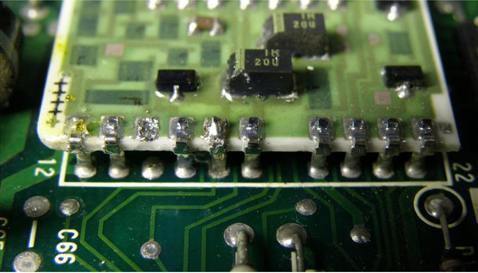
5. Retaining the zener diode is still recommended, as the opamp may not protect against over voltage from the AFM if it occurs. It will need to be moved to the input side of the ECU
