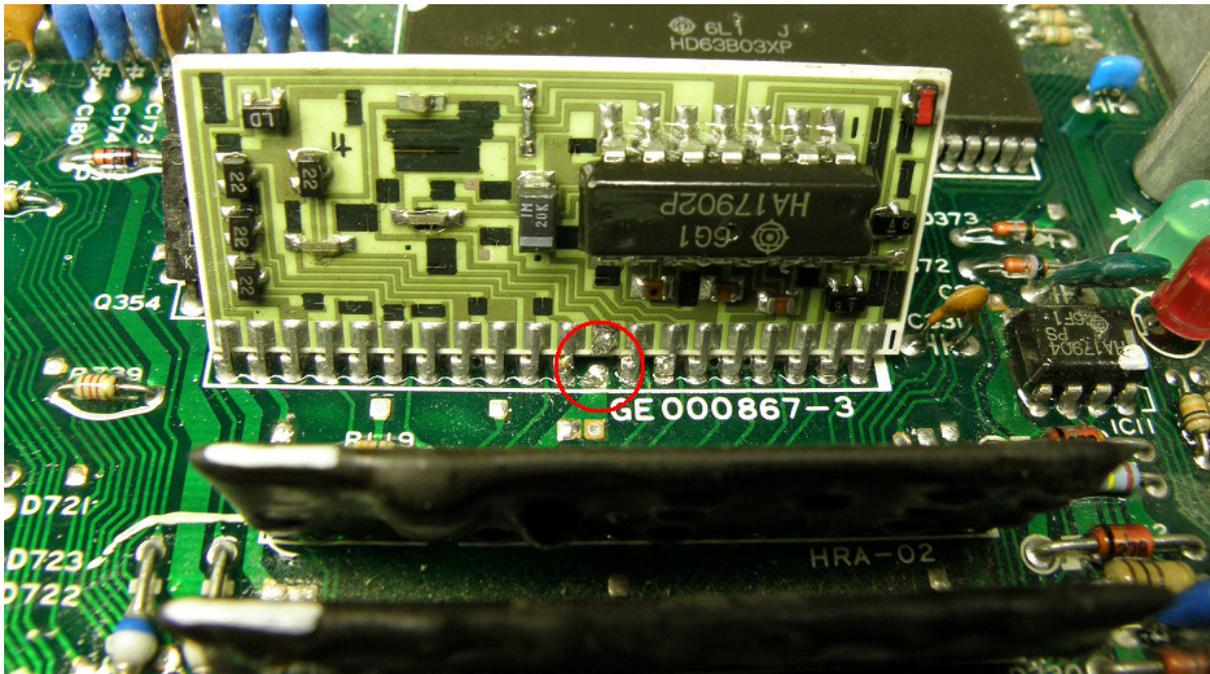
2. Remove pin 9 from the board to the ECU. This is the voltage line to the opamp. Do this by removing solder on the reverse side using a desoldering gun and then heading the front side with a soldering iron and prying away with a small screwdriver or tweezers.
