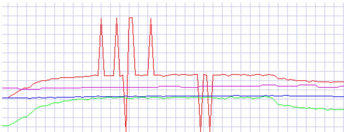
The removal of the opamp from the circuit has affected filtering of the ECU and occasional spikes in the fuel injection could be potentially noticed. In the log above TP was not affected, so the map points accessed were not changed.
