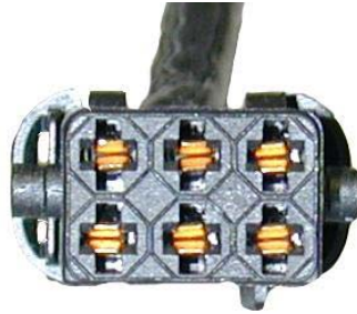
Figure 7. UEGO Sensor connector Latch Removal
