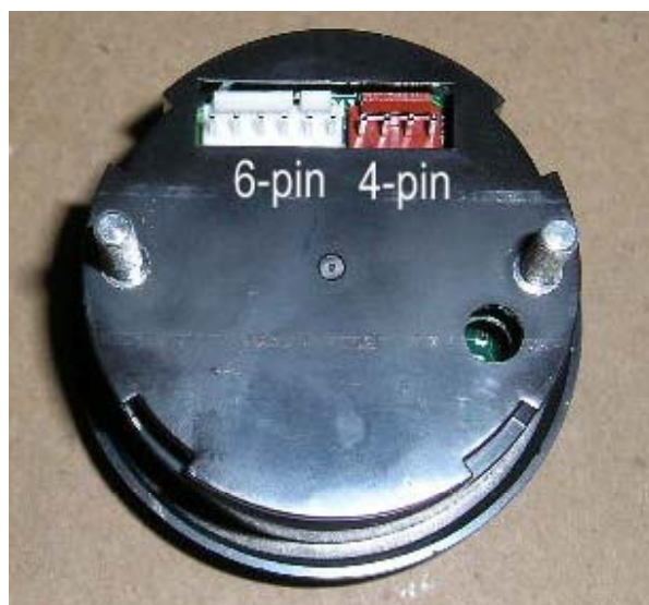
Figure 4. Gauge Side Harness Connections
