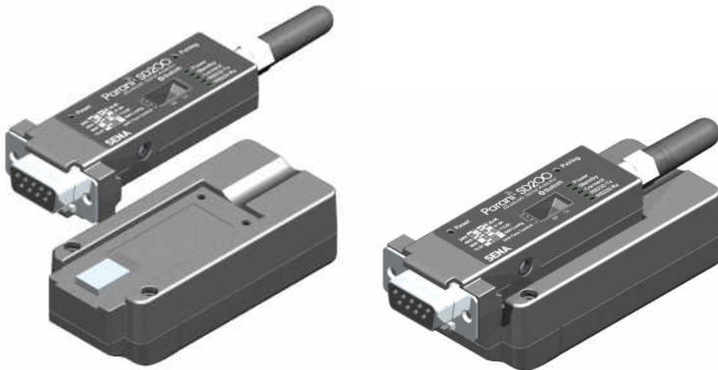
Figure 2-5 Attaching Batter Pack to Parani-SD200
