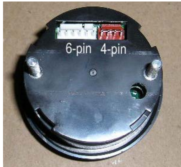
Figure 4. Gauge Side Harness Connections
